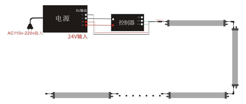
Note: The above wiring diagram is normal wiring diagram. The specific wiring diagram depends on the load capacity of the controller and the actual situation wiring
