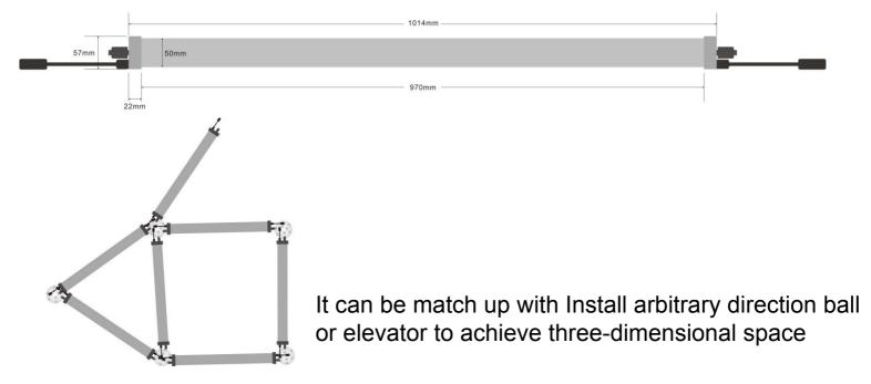
Note: The above is chart of one meter, normal size we have 1.5M and 0.5M, It also can be customized.
