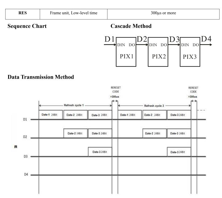
Note: D1 is the data from MCU, and D2, D3, D4 are from Cascade Circuits.
